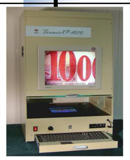
**ForensicXP–4010** is the only commercially available forensic digital imaging spectrograph for large-scale document examination. The instrument together with original 2D/3D processing software represents a new generation of nondestructive tools for authenticity determination of different types of documents and handwritings. The system, based on examination of the objectively measurable physical parameters, is aimed for forensic document experts involved with questioned document inspection.
